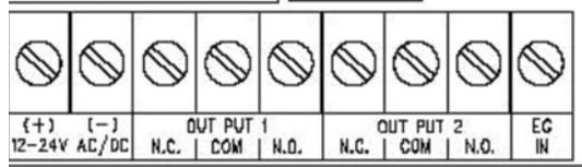
2. **Connect the OUTPUT 1** N/O and COM to OPEN contacts in the operator (see operator manufacturer's manual for proper terminals)
