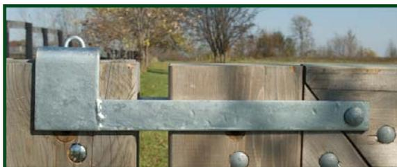
Latch two gates together. Heavy duty construction. Hot dipped galvanized finish or black powder coat over galvanized. Fits gates 2 3/4" to 3 1/8" thick. Notch in throw over gate loop closes over staple on plate. Can be locked with a padlock or snap fastener (essential when used with livestock). Includes fasteners and staple on plate. Padlock and clip not included.
