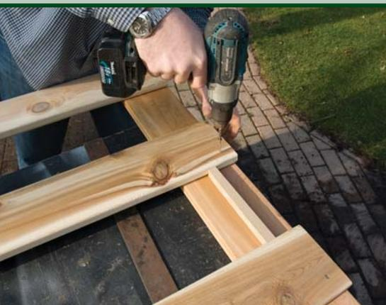
**3** Measure distance between top and bottom board. Place two other rails and space equally. Cut two scraps to ensure the accurate placement of the horizontal rails.
