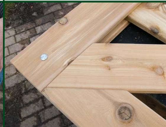
**8** Lay top rail and diagonal in place ensuring a good fit. Install a 1.5" wood screw into each (screwing up from the bottom) to hold top rail and diagonal in place.
