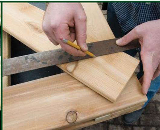
**7** Using a straight edge mark pencil line on diagonals even with inside edge of stiles. Mark top and bottom. Remove top rail and diagonal. Cut along pencil marks.
