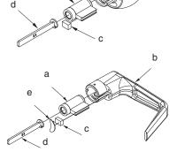
H-3 Assemble the required tailpiece (d) supplied with your KIL/KIK cylinder. All tailpieces must be installed vertically as shown for proper installation.
