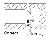
N-2 Mark locations where the gaps are approximately \%" (5 mm). Make sure these locations are free from grease and dust. Peel the bumpers (c) (supplied) from their protective backing without touching the adhesive surface and stick them on the marked locations. Note: Allow 24 hours for adhesive to set
