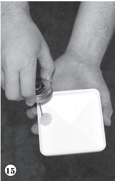
15 Apply a moderate amount of PVC adhesive on the inside of the roof beam end caps.
