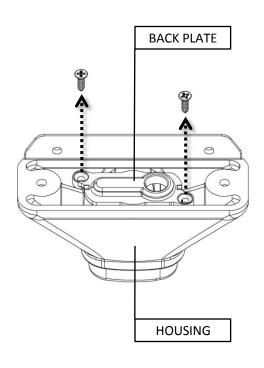
Step 2: Remove Button from Housing.
