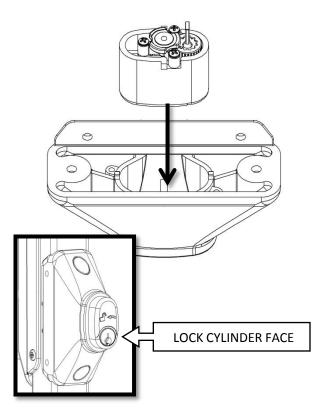
Step 3: Using two Philips head screws, screw Back Plate into Housing as shown.
