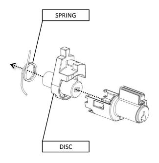
Step 4: **A**. Un-clip the hook on the Lock Cartridge and open as shown.
