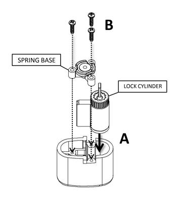
Step 2: Insert Button into Housing, checking that Lock Cylinder Face will be at the bottom when mounted on post.
