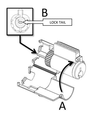
Step 2: Install Spring and Disc into cartridge.
