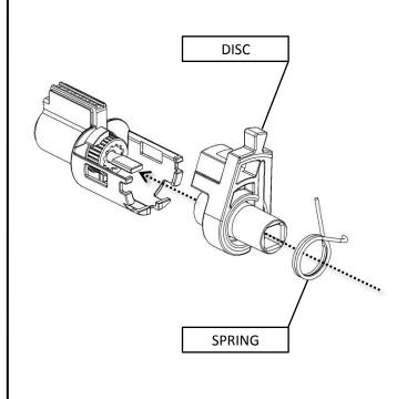
Step 3: Insert Lock Cartridge assembly partly into Body until position as shown (!)
