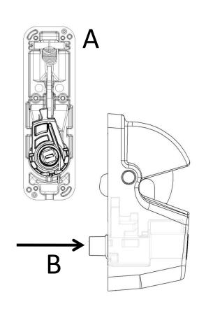
Step 7: Check that the face of the Lock Cylinder is flush with outer Body and not at an angle.
