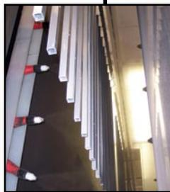
**STEP #8:** A convection oven completes the dry-off process.
