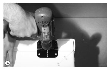
Holding the lid tight to the back wall of the bed predrill and fasten each hinge with screws.
