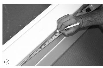
Determine the center of the box and make a mark for position on the top front of the lid.
