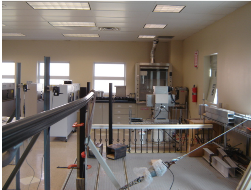
Photo No. 3 Vertical Concentrated Load Test at Ends of Contour Handrail (Brackets)
