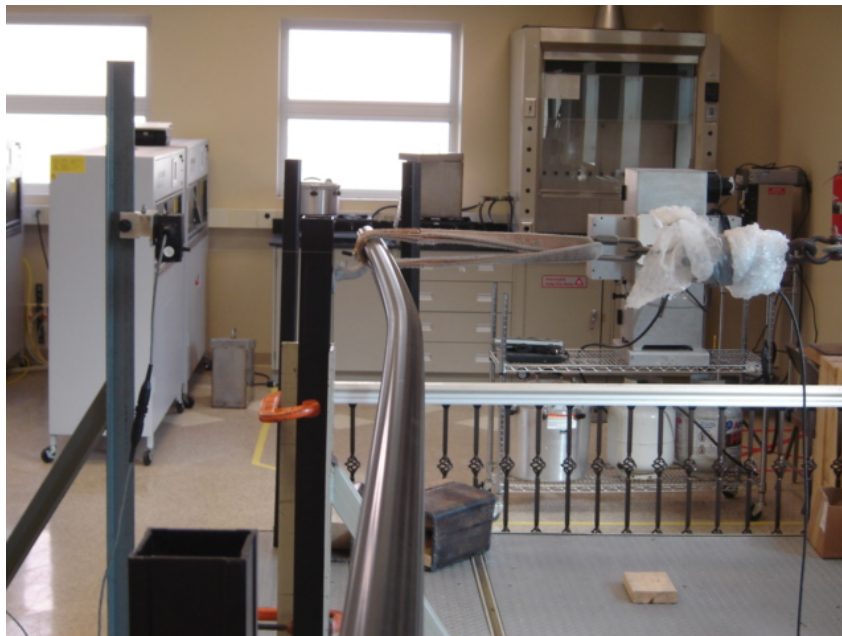
Photo No. 2 Horizontal Concentrated Load Test at End of Contour Handrail (Brackets)
