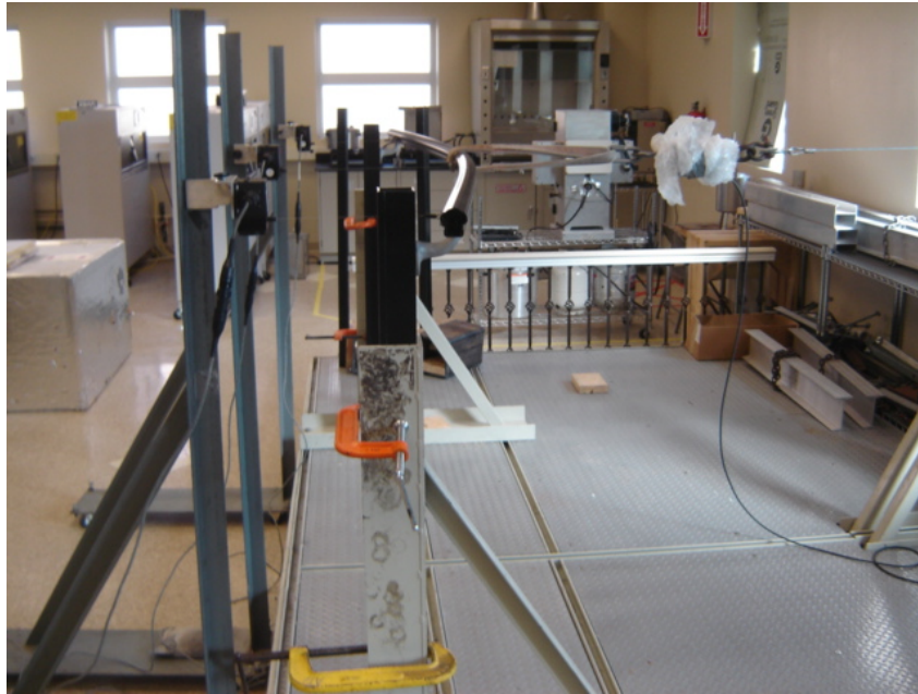
Photo No. 1 Concentrated Load at Midspan of Contour Handrail
