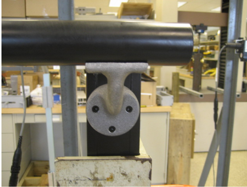
Photo No. 7 Typical Die-Cast Aluminum Bracket for 1-1/2 in Diameter Handrail
