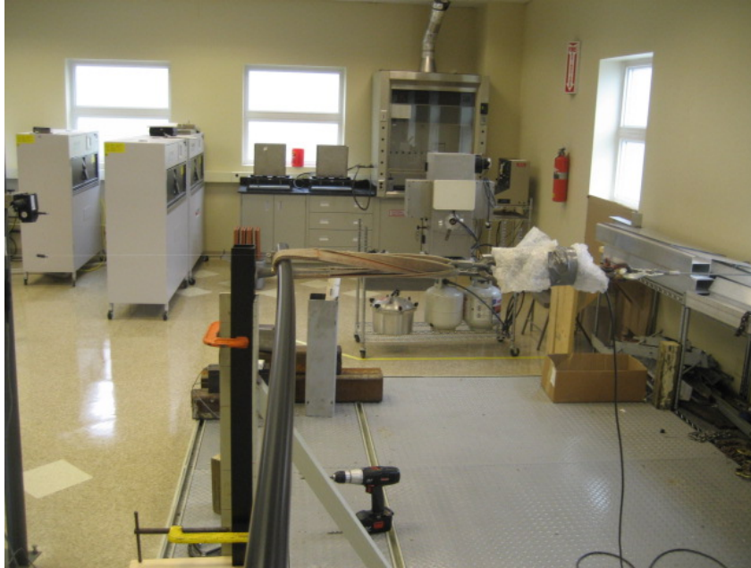
Photo No. 5 Horizontal Concentrated Load Test at End of 1-1/2 in Diameter Handrail (Brackets)
