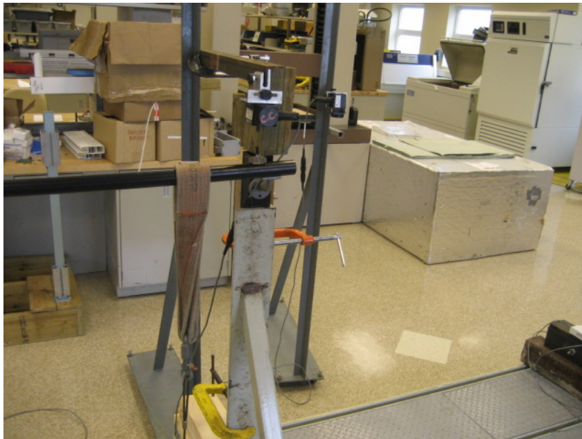
Photo No. 6 Vertical Concentrated Load Test at End of 1-1/2 in Diameter Handrail (Brackets)
