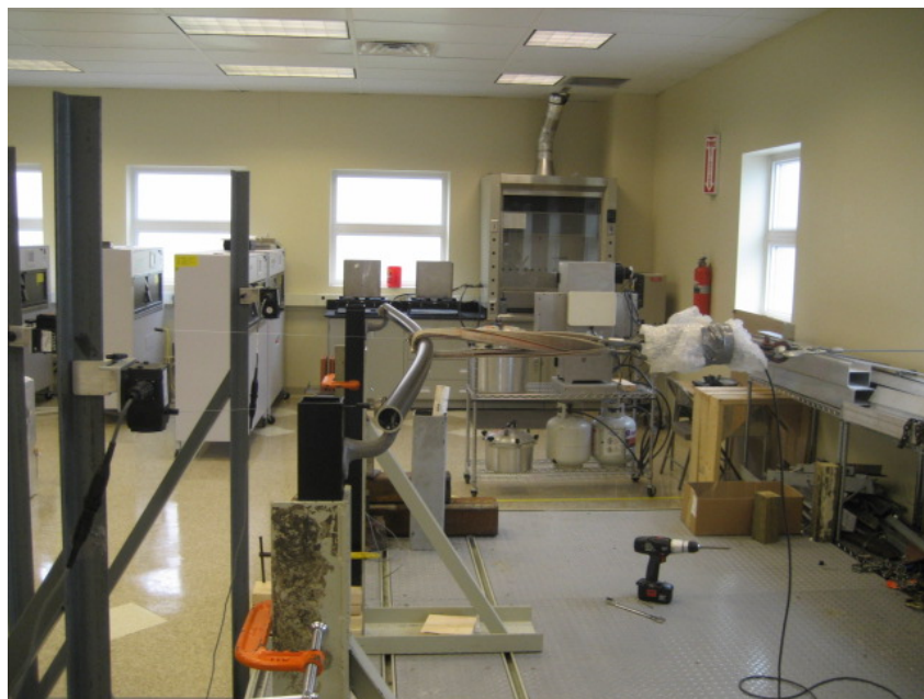
Photo No. 4 Concentrated Load at Midspan of 1-1/2" Diameter Handrail
