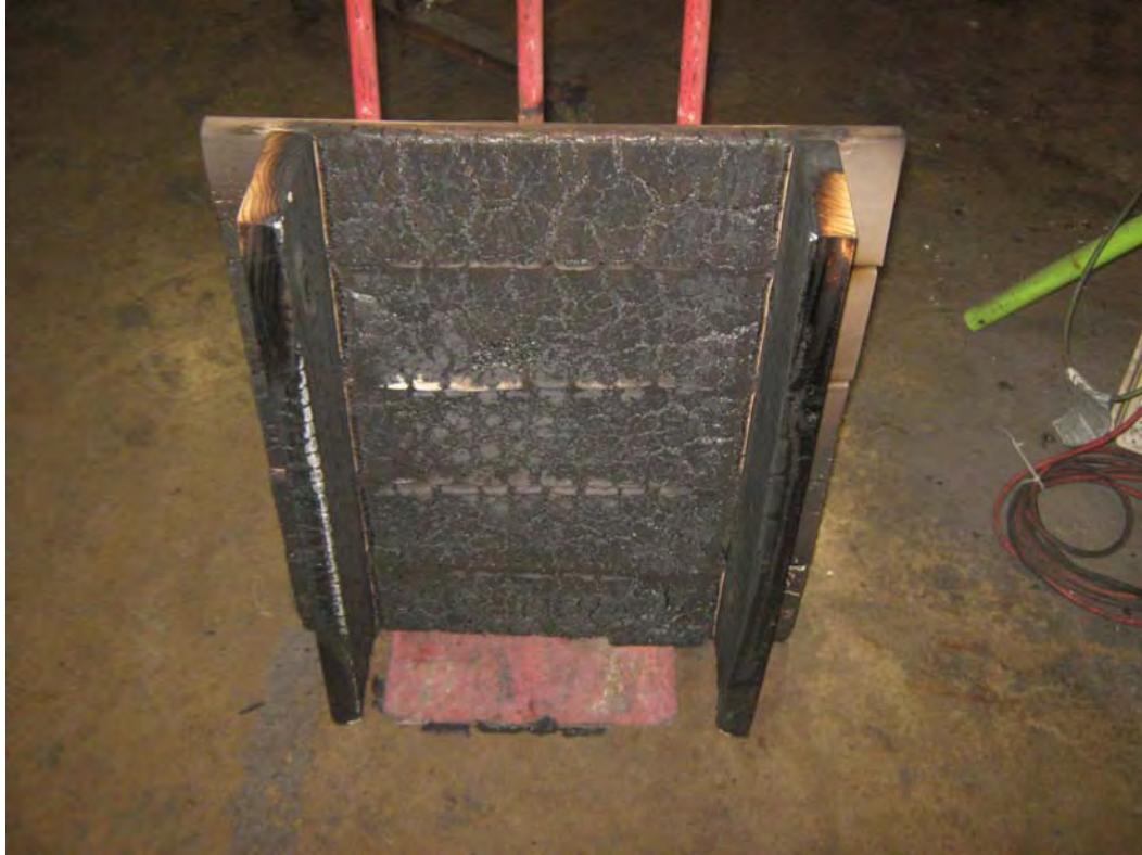
Post-test damage, underside
